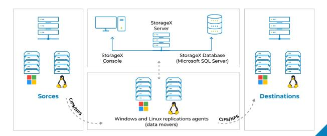
The StorageX server and replication agents can be installed on virtual or physical servers. StorageX replication agents do the heavy lifting, moving file data based on policy and configuration information provided by the StorageX server. The StorageX server and StorageX Console run on Windows 2008 R2 or later. StorageX replication agents run on Windows 2008 R2 or later or Red Hat Enterprise Linux 6 or Red Hat Enterprise Linux 7.
