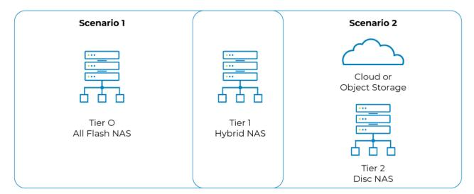
Optimized for higher performance environments storing 80% of data stored on Tier 1 hybrid NAS with 20% of data (most active) stored on Tier 0 all flash NAS. Optimized for storage efficiency storing 20% on Tier 1 hybrid NAS, 40% on Tier 2 Disc NAS and 40% in Cloud Object Storage for archive data
